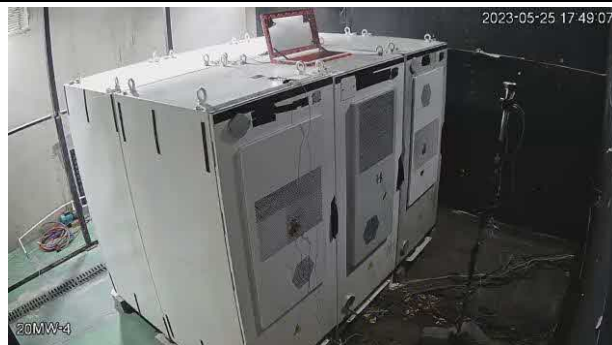
Figure 16: 3 rd cell venting (Time at 17:49)
