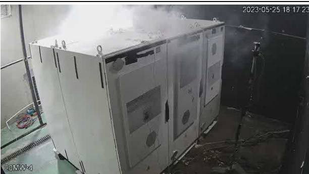
Figure 18: 2 nd cell thermal runaway (Time at 18:17)
