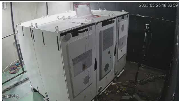
Figure 21: 5 th cell venting (Time at 18:32)
