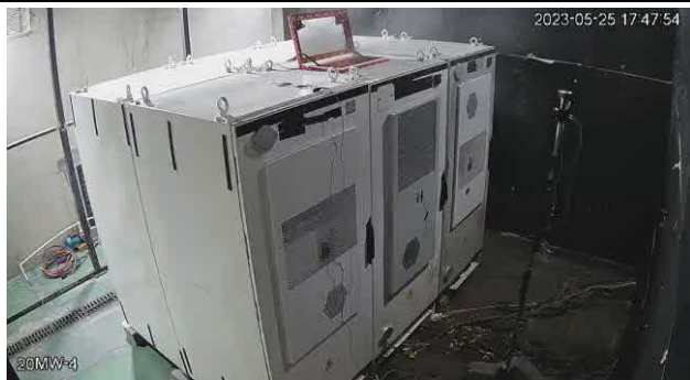
Figure 15: 2 nd cell venting (Time at 17:47)
