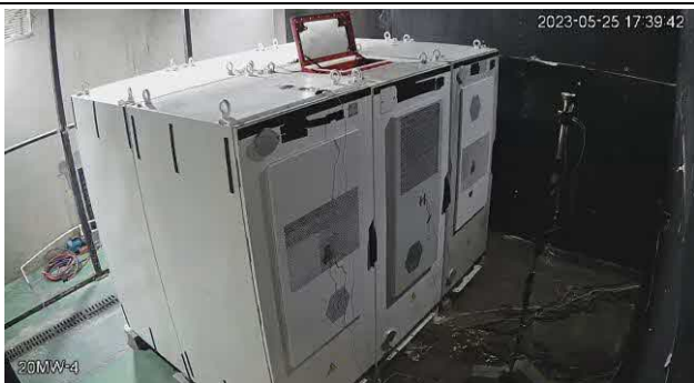
Figure 13: Ventilation valve (inlet) and window unfolded (Time at 17:39)
